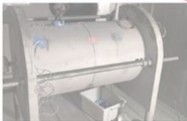
Figure 4. Welded pipe set-up.
