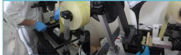
BOBIPREG (3X pre-preg machine) Kevlar® tape with 3X resin impregnation
