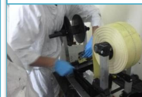
Tape impregnation using BOBIPREG & R4D-S wrapping (step 4)
